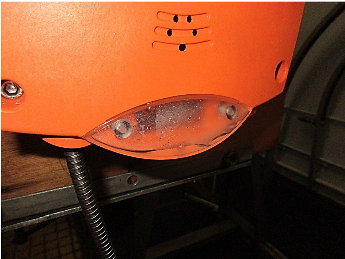
Presence of water inside the flash lamp external diffuser after test for the protection against penetration of water.
