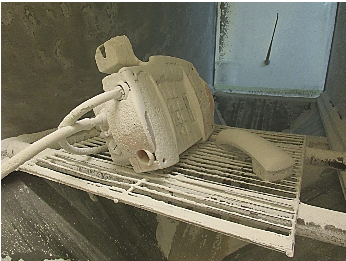
Equipment before and after test for the protection against ingress of dust.
